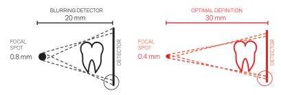
Increased X-ray parallelism and an incorporated collimator allow the RXDC to achieve a source-to-skin gap of 30 cm. The RXDC provides pin-sharp, precise images with outstanding detail.
